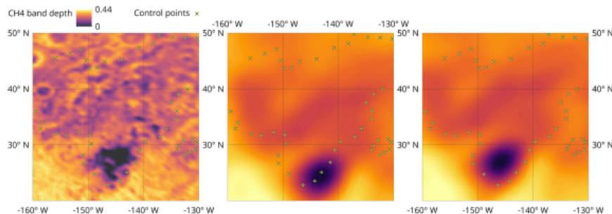
Validating LEISA registration: a) high-resolution data; b) misregistered low-resolution data; c) registered low-resolution data
