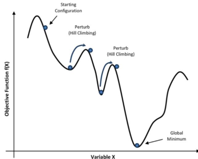
Schema showing the concept behind simulated annealing (Ghasemalizadeh et al., 2016)
